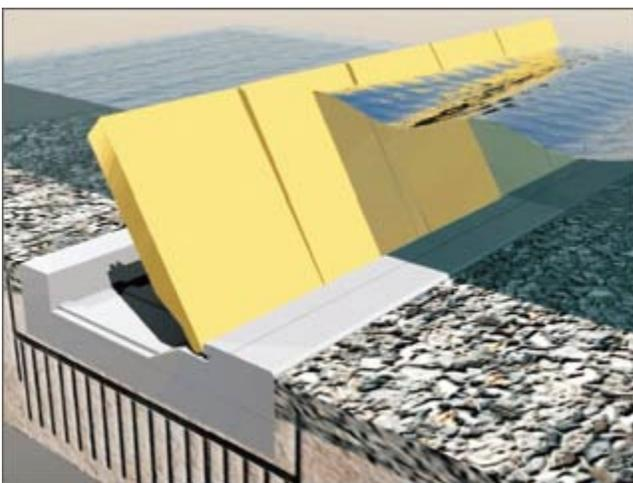
**Figure 25. Flap gate to be used in Project Moses at Venice, Italy**
