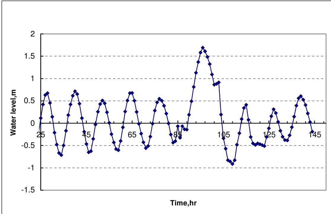
**Figure 13. With two barriers closed and the East River open during Super Floyd, the peak water level is higher than if all three barriers were open.**
