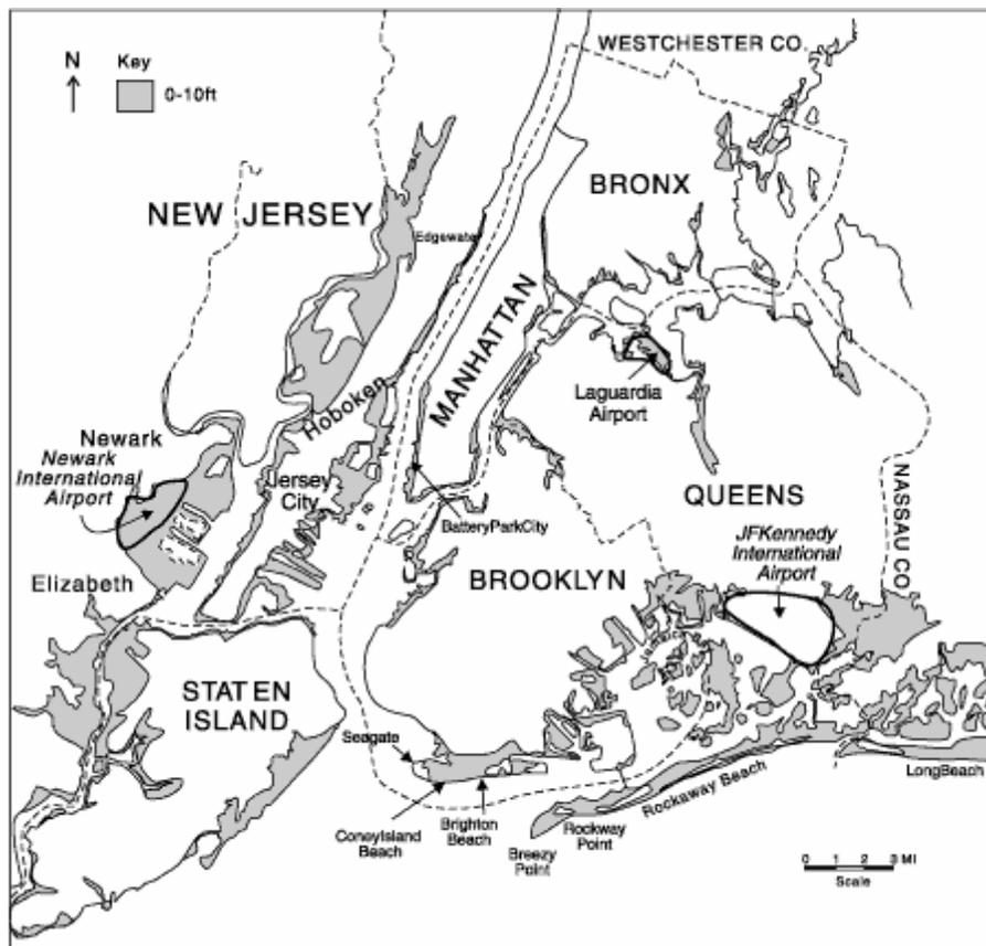
Figure 1. The 100-year flood, shown shaded, covers 260 square kilometers in the metropolitan region, about half of which can be protected with storm surge barriers. Source: V. Gornitz, in C. Rosenzweig and W.D. Solecki, *Climate Change and a Global City*, Columbia Earth Institute, July 2001.
