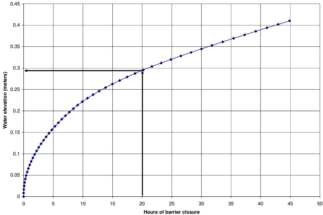
**Figure 18.** Considering only the storage volume above the upward sloping Hudson River, the rainfall runoff crest would raise the water level behind the barriers less than 0.3 meters during the 20 hours that they would have been closed for Tropical Storm Floyd, and less than 0.4 meters in 40 hours.
